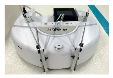
...Graphic 1. The robot that was used in the experimental assembly with the sensor-mount clearly visible
