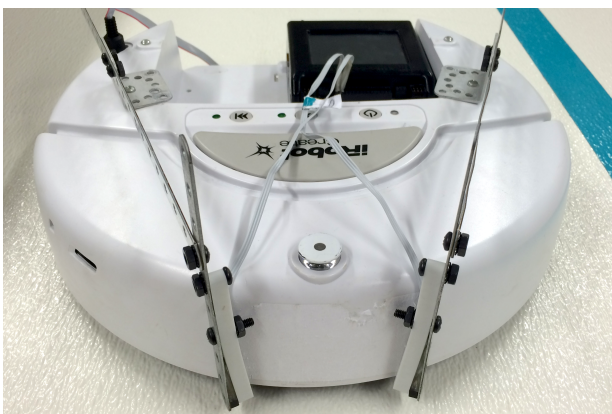
Graphic 1. The robot that was used in the experimental assembly with the sensor-mount clearly visible
