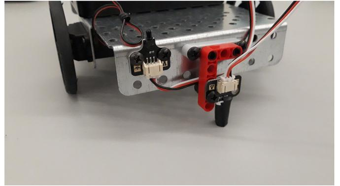
Fig. 5: A simple robot made of Botball parts with a shielded IR-sensor
