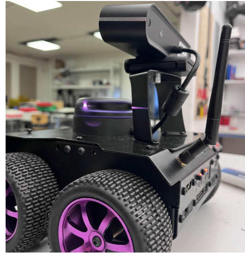
Figure 1: The ROSbot, front left side, close up with no changes or edits to how the original robot looks like
